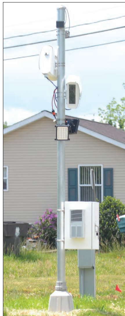
CHARLENE SHARPE/BAYSIDE GAZETTE The speed camera on Flower Street are pictured this week.
